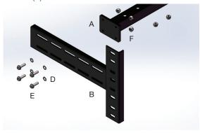
Place four (4) Bracket Bolts (E) with four (4) Lock Washers (D) through the slots of the Outer Headboard Bracket (B) and into the holes of the Inner Headboard Bracket (A). Use four (4) Locking Nuts (F) to secure the brackets in place, but loose enough to allow adjustment.
