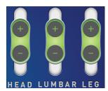
Tap and slide\* the +/button for the **Head**, **Lumbar**, or **Leg** to adjust
